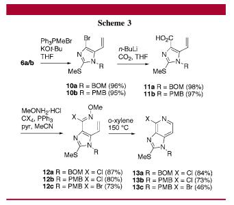
and upon treatment with carbon dioxide, they produced carboxylic acids **11a** and **11b**. Applying the methodology of Kikugawa, we transformed BOM-protected compound **11a** directly into *N*-methoxy imidoyl chloride **12a** in good yield.<sup>10</sup> Similarly, the PMB-protected acid **11b** was converted into both the *N*-methoxy imidoyl chloride **12b** and the corresponding bromo compound **12c**.
